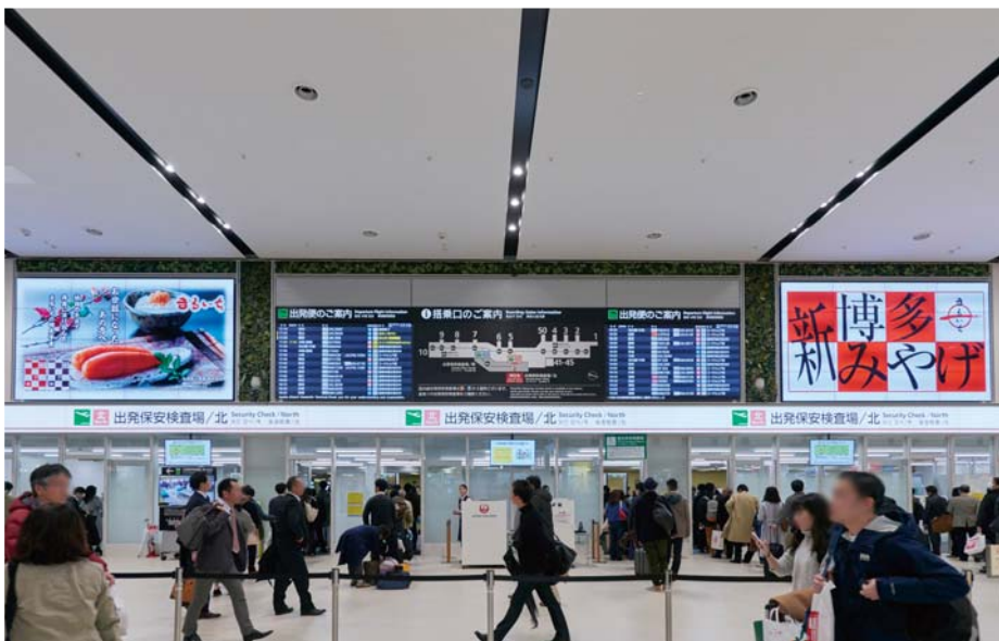
▲ Four vertical screens x four horizontal screens were installed with an aspect ratio of 16:9, the same as an ordinary wide-screen display. Advertisers were pleased with the excellent color reproduction of the IPS LCD panel.
